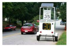
to detect what time of day the most number of people are speeding in an area so that additional enforcement can be placed there if needed. The boards basically run themselves and can be powered off of batteries or by solar power. The portable boards work well for moving to different areas where speed is of concern. Permanent boards can also be installed at problematic locations. One concern with these boards is that it may encourage certain groups of drivers to speed if not monitored.
