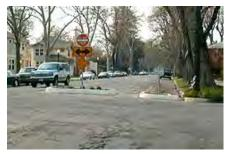
Half closures are put in place to block a single lane of traffic. They can be used to prevent vehicles from entering a road but still allow vehicles to exit the road. This is an effective means of limiting traffic on a roadway and also limiting turns off of the intersecting roadway. Half closures are generally made by extending the curb or placing a barrier to block entry. Ample signage must be put into place to alert drivers to the partial closure. Half
