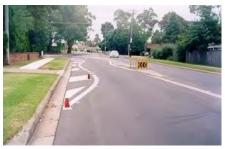
Pavement markings can be used for anything from onstreet parking, to accentuating already existing features, to creating new features. Using pavement markings to indicate areas where on-street parking would occur creates a safer parking environment and also directs traffic in the area. A slight speed reduction may occur if the travel lanes are narrowed due to the markings. When pavement markings are used to accentuate already
